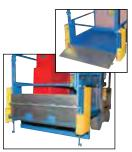
**Automatic Fold Down** Ramp, series WP-AFR, allows you to roll tool boxes on and off the Work Platform. Ramp automatically rises when the unit is lifted off the ground and lowers when work platform is lowered. Option comes standard with a front chain gate. (This option is not compatible with the WP-CA caster option.)
