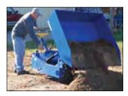
Briggs & Stratton gas powered motor and a traction drive system for overcoming the roughest of areas. Durable steel construction for added strength and long life. Power dump capabilities for smooth, ergonomically friendly unloading, and an emergency shut-off release for extra safety. An optional Line-X inside hopper coating available upon
